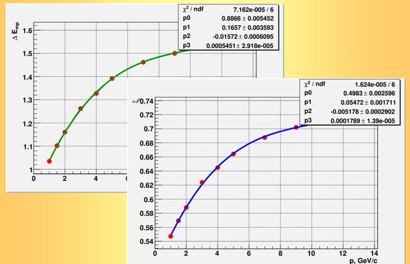
Figure 3: Dependence of the  $\Delta E_{mp}$  (green line) and  $\xi_i$  (blue line) against the momentum and its approximation by a polynomial of the third degree
