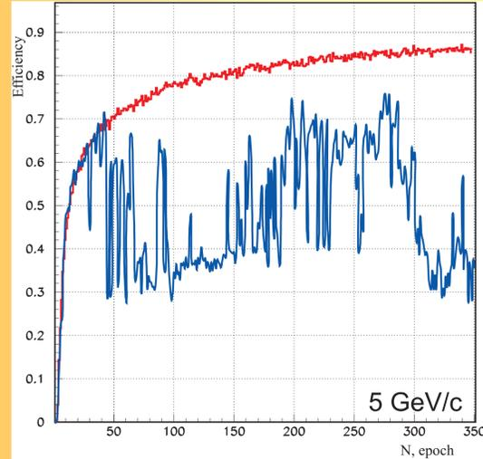
Figure 2: The efficiency of  $e/\pi$  identification by the MLP for original (blue curve) and transformed (red curve) samples for  $e$  and  $\pi$  with  $p = 5 \text{ GeV}/c$
